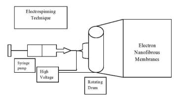
Fig. 2 Electrospinning Technique for synthesis of polymer composite
