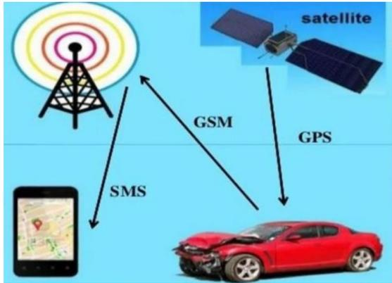
The above given is the system model. This intelligent accident identification and location display system will be fitted the cars which will work as-
