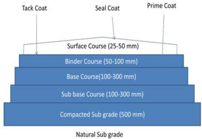
**Figure 1 Layers of Flexible Pavement**
