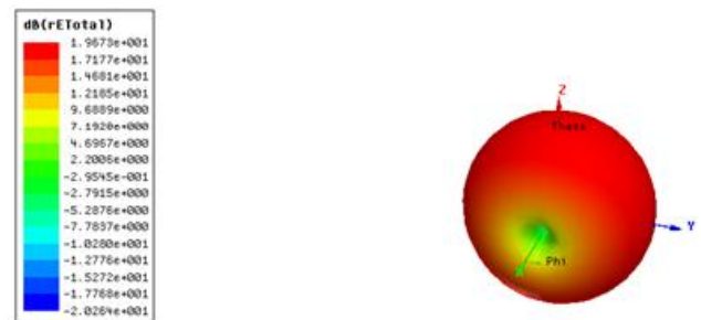
Figure 10. Simulated Gain of antenna for ground plane (Lg) 8mm
