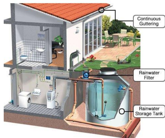
Figure 2 Rooftop rain water harvesting
