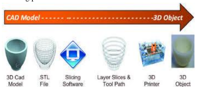
Figure 1.1 Principle of 3d printing
