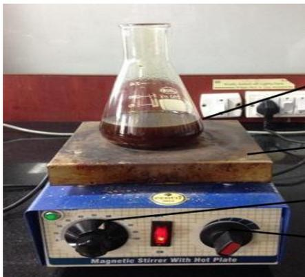
**Figure 2 Pre heating of neem oil on magnetic stirrer with hot plate.**
