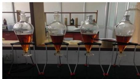
**Figure 4.2: Final methyl ester of neem oil formed after the hot water washing.**
