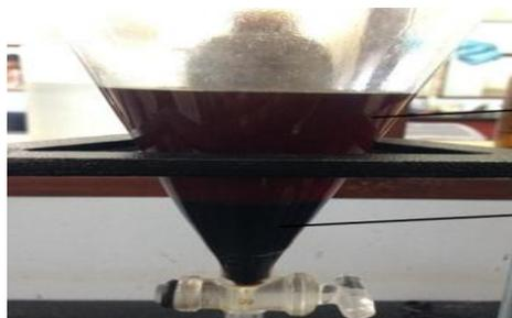
**Figure 4.1 Separated layers after base catalyzed stage.**
