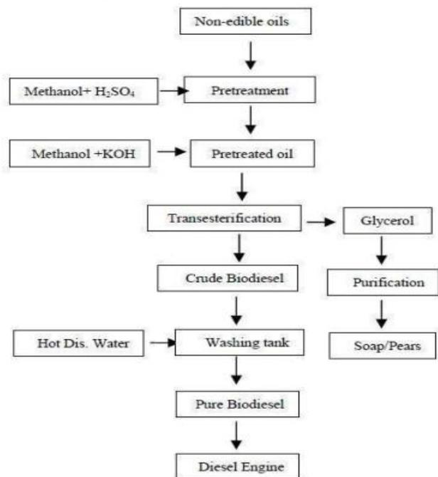
**Figure 1 Process of bio diesel**
