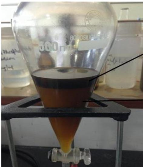
**Figure 3: Two layers formed after the acid catalyzed stage.**
