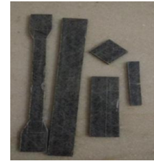
Figure:10 Hybridization of basalt with E-glass fiber reinforced Epoxy Composite
