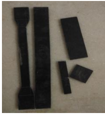
Figure12 hybridization of basalt/E-glass fiber with 6g of graphite powder reinforced Epoxy Composite
