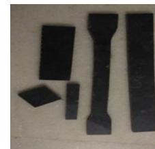
Figure 11 hybridization of basalt/E-glass fiber with 3g of graphite powder reinforced Epoxy Composite
