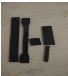
Figure13 Hybridization of basalt/E-glass fiber with 9g of graphite powder reinforced Epoxy Composite
