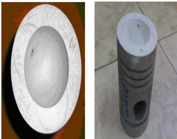
2.Photographic views of base engine and TiO2 Coated piston
