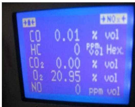
fig 3. Photographic view of the exhaust gas analyzer showing a sample results
