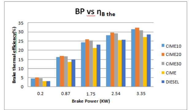
**FIG. 3 BP v/s  $\eta_B$  the diagram**
