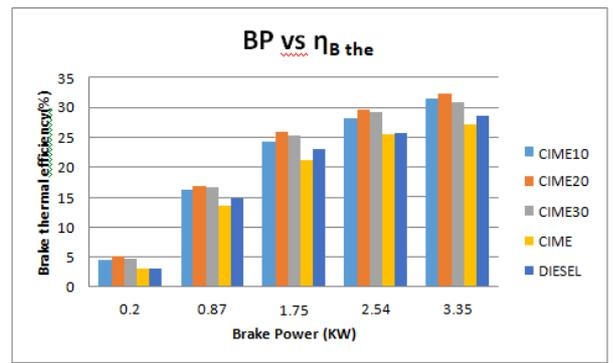
**FIG. 3 BP v/s  $\eta_B$  the diagram**
