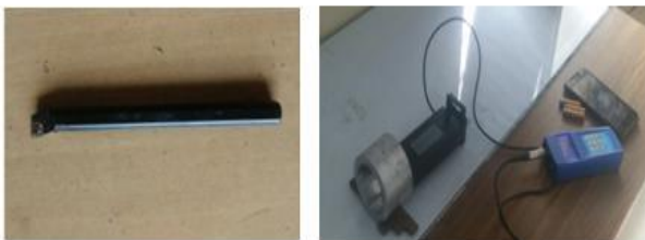
Fig.5.(a) boring bar (b) surface roughness tester
