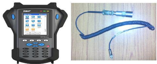
Fig. 4(a) FFT analyzer (b) Accelerometer
