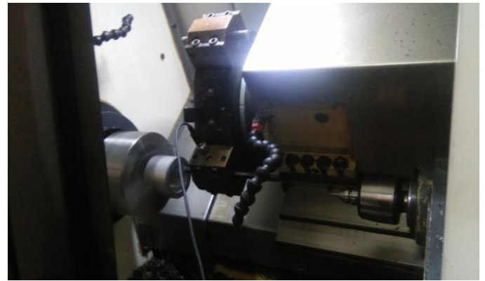
Fig. 4 Experimental set up for boring operation
