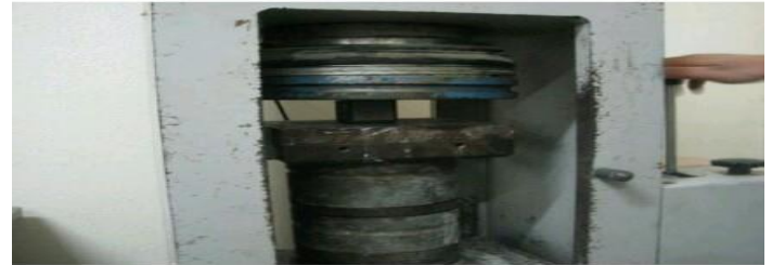
fig.6 Cube during compressive test
