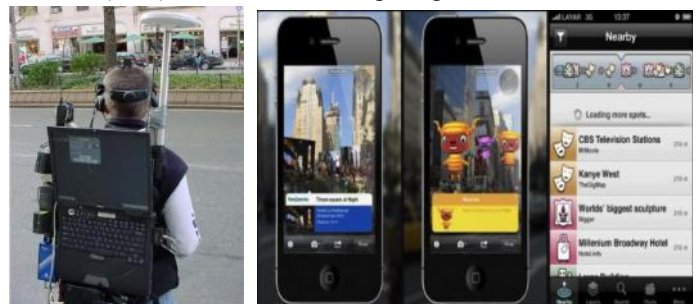
Figure 2: Mobile AR: (a) user with Mobile AR system backpack; (b) example of AR application that uses mobile devices.
