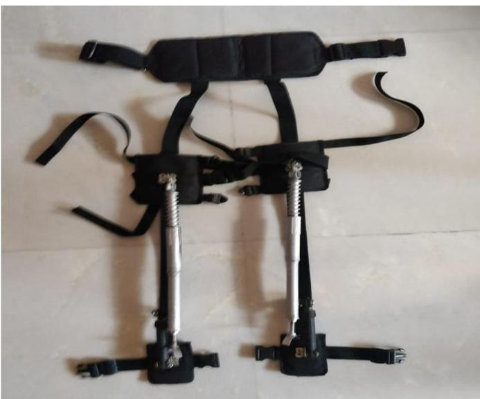
our concern when design this chair is to reduce muscle cramp due to standing for a long time so, we expected the user will only move in short distance. Next, it is proven to be suitable with any range of height because the dimension that were used has consider the average height of Asian people.
