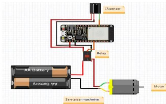
An automatic hand sanitizer system was created, and it will be given in two stages, with the first presenting the instrument construction and the second discussing the control portions. The goal of this project was to improve people's access to gadgets by utilising the flexibility of pumps.
