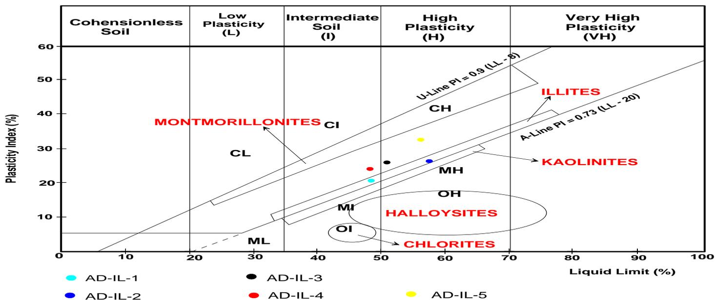
Figure 3: Casangrade Plasticity Chart and Corresponding Clay Groups of the Sampled Soils [29]
