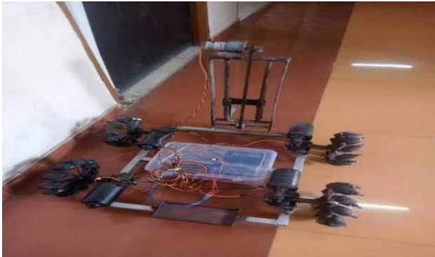
Fig. Final model of Mecanum wheel for industrial purpose
