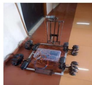
Fig.-Final model of Mecanum wheel for industrial purpose
